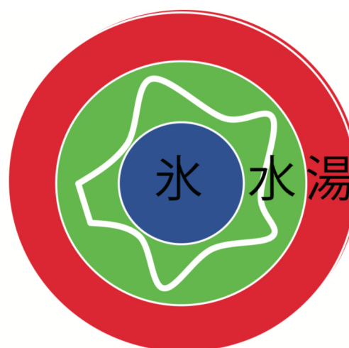
図12 dishpan実験の模式図
